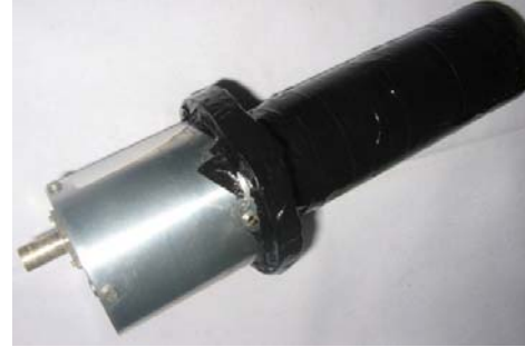
7: Assembled PMT with Voltage Divider
