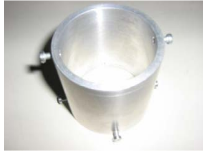
2: Housing for PMT Voltage Divider
