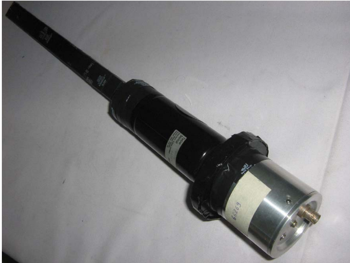
Fully Assembled Narrow Scintillator Finger Paddle coupled to Photomultiplier Tube.
