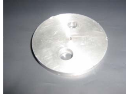
3: Plate for mounting HV & Signal Connectors
